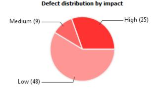
From this pie chart, you can obtain a graphical visualization of the defect distribution by impact. You can find at a glance whether the defects that Polyspace Bug Finder found in your code are low-impact defects. For more information on impact, see "Classification of Defects by Impact" on page 5-7.
